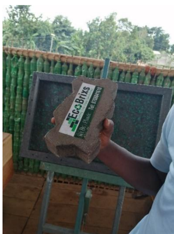
Image 14. Brick, black board and frame from plastic at Ecobrixx in Masaka, 17.5.2021, a.p.
