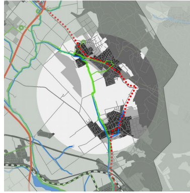
Figure 5: A cycle route section in the regional plan alongside a main road versus a greenway section alternative alongside a traditional trail versus train for regional cycle route
