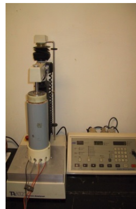
Figure 2. SMS TA-XT2 precision penetrometer and coaxial test cell
