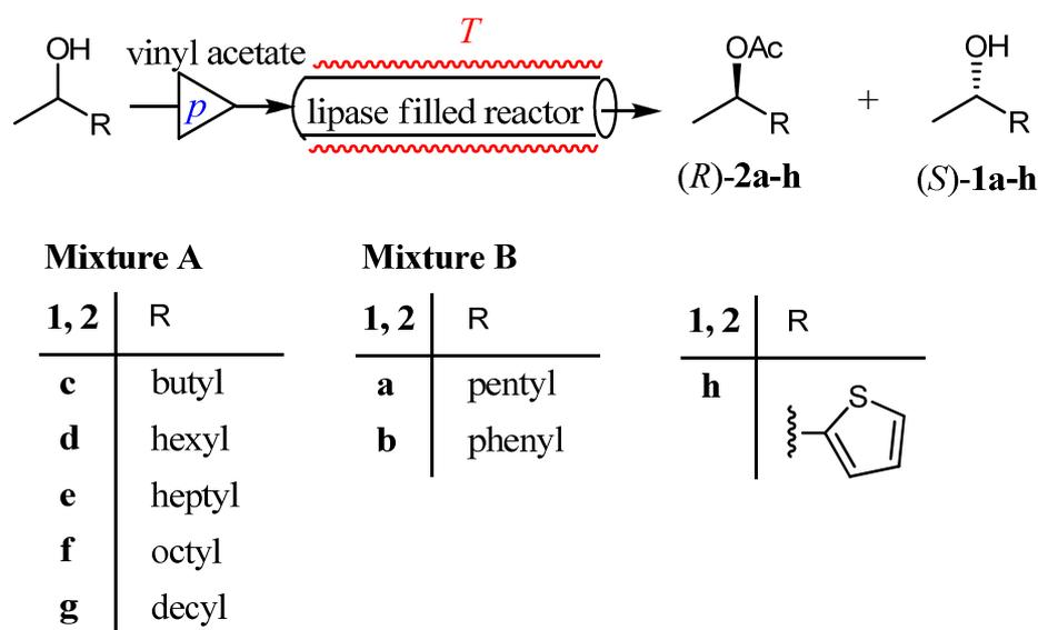
**Figure 26.** Multiple substrate (*rac-1a,b* and *rac-1c-g*) and single substrate (*rac-1h*) kinetic resolutions in continuous-flow reactors. [▷: pump; ~: temperature control unit].
